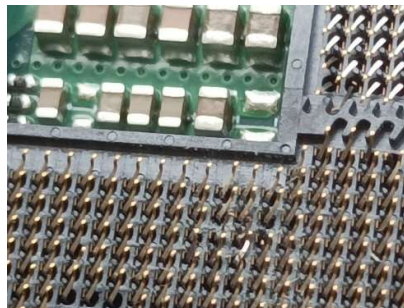
Figure 21: Bent Pins on Router Socket
